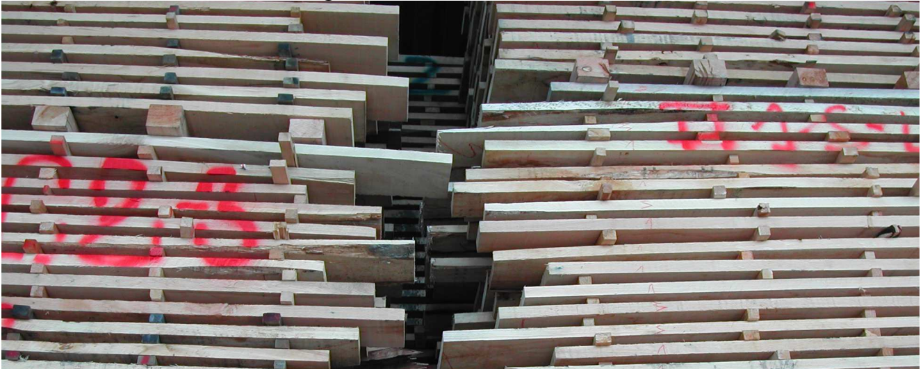
BEFORE – very poor kiln sticker alignment
